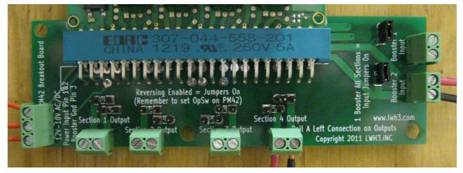
The breakout board eliminates soldering connections to the card edge or card edge adapter of a PM42 circuit breaker/reverser board.
